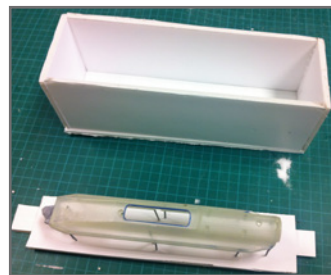
A silicone mold pattern and mold box are ready for pouring.
