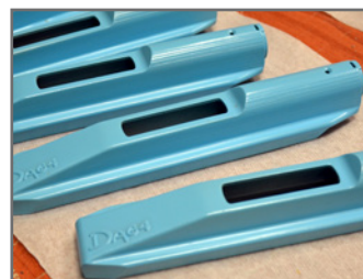
Raw urethane castings from a silicone mold.
