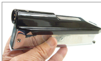
Concert-ready harmonica with silicone-molded amplifier.
