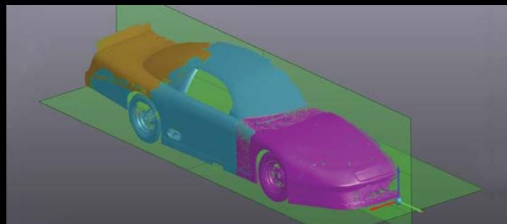
VXmodel features highly flexible tools required to align a 3D file to the coordinate systems using datum/entities suited your design requirements. VXmodel also enables users to align meshes together or a mesh on a CAD model.
