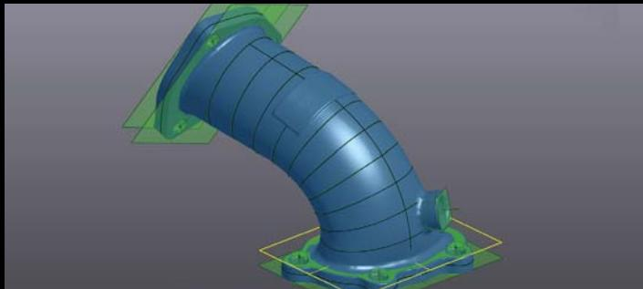
Use a 3D scan as a reference for a design by extracting all the useful information from the mesh. Segment the mesh into all of the primitive entities required to complete the design in a CAD software with VXmodel's highly flexible and user-friendly interface.
