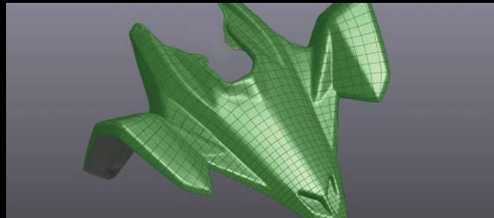
VXmodel enables you to easily generate NURBS surfaces for characterizing freeform surfaces for later use in your CAD software. With its powerful algorithm and intuitive interface, the auto surface function generates high-quality NURBS surfaces and a well-organized patch network.
