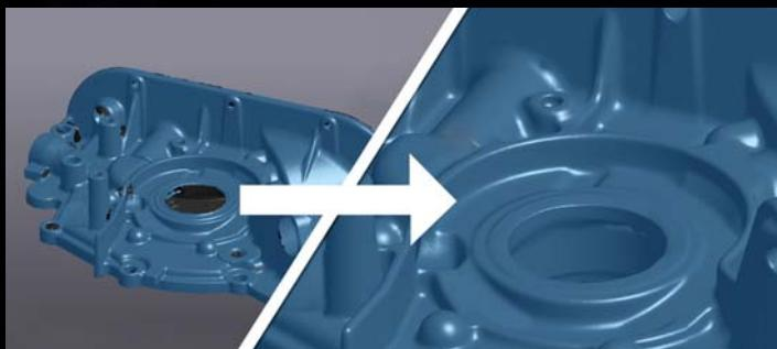
VXmodel offers simple, yet powerful, tools required to prepare the 3D scan mesh for reverse engineering or 3D printing.
